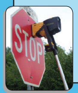
A retroreflectometer is placed against each sign to measure sign retroreflectivity. Signs with below minimum levels should be replaced.
